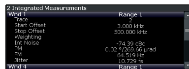
Figure 3-2: Custom integration range results (frequency range from 3 kHz to 500 kHz, applied to trace 2)
